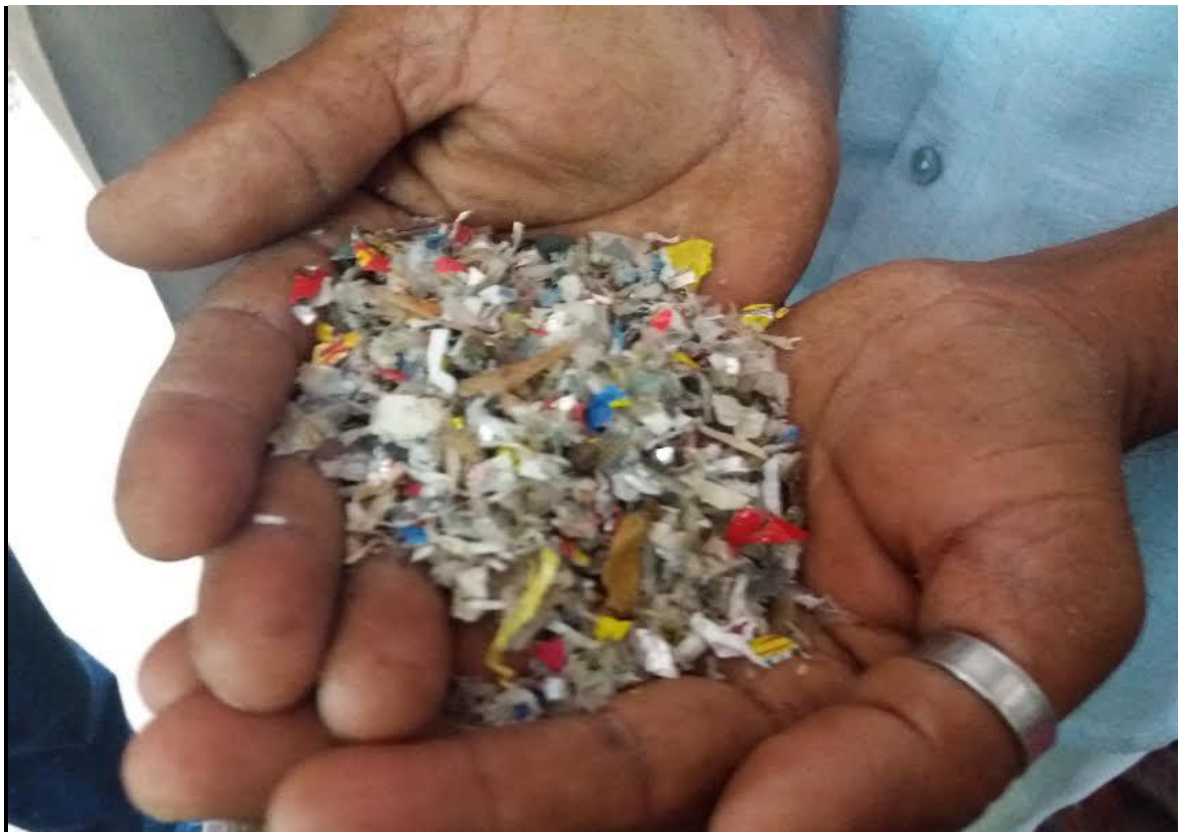
Shredded Pieces (8mm) of Polyethylene Covers; ready to use in BT roads.
