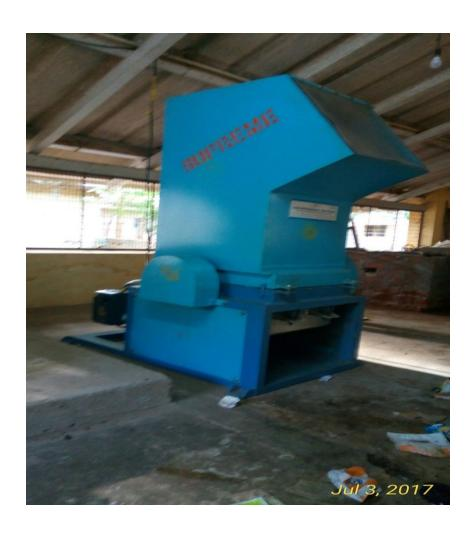
Motor :10HP/1444 RPM/440 V
