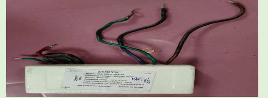
Surge Protection Device (SPD)
